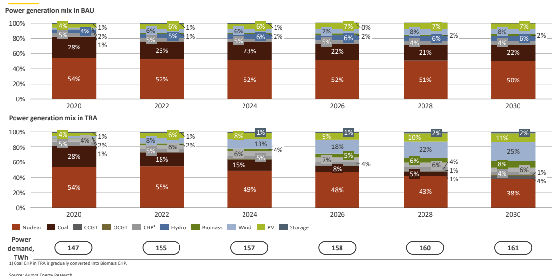
Figure iii.: Power generation mix in BAU and TRA
