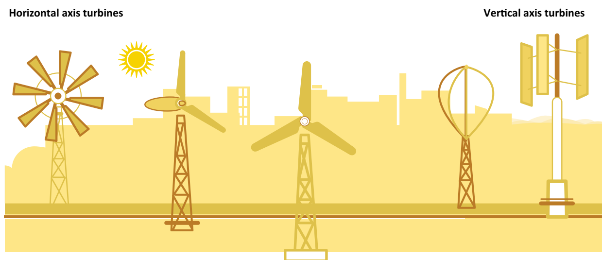
Figure 7.5. EWEA early wind turbine designs
